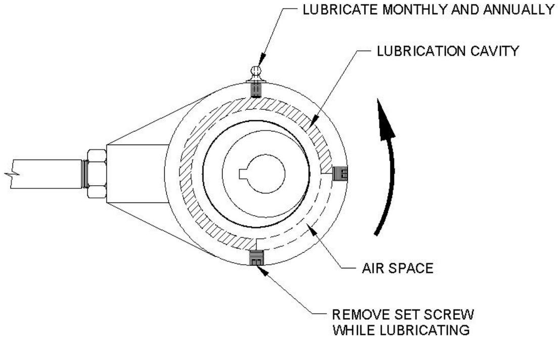
The function of the unit is designed specifically to provide maximum separation of berries and MOG. If the performance is poor then it may become necessary to ensure that the motor and eccentric bearing are rotating in the proper direction.
