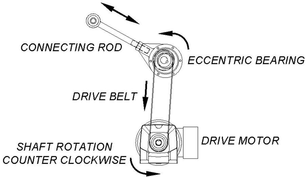
If the rotation is not as indicated, correct by swapping the two power leads at the drive motor junction box.
