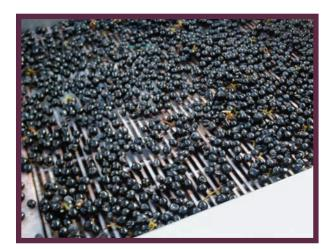
averaged 6 tons/hour for the duration and allowed secondary hand sorting as an unplanned bonus. Our final production units will process at 8-10 tons/hour.
