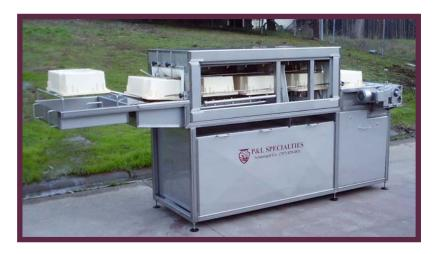
stubborn material. The second stage features a high temperature, high pressure rinse to ensure cleanliness. Both stages are internally screened and filtered to assure consistent results and minimize water consumption.
